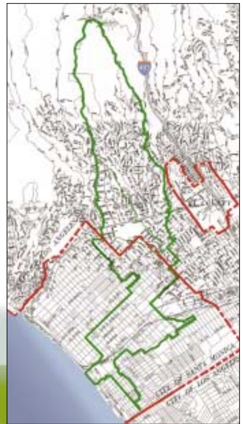
The image at right shows the total drainage area (in green) for the Pico-Kenter storm drain within the City of Los Angeles extending into the Santa Monica Mountains. The LA County portions (in red) show the cities of Beverly Hills and Santa Monica.
